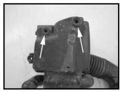
Step 10 Remove the factory grommet from the air box. This will be reused on the next step.
